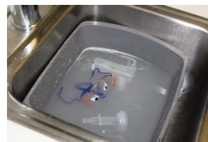
11. Turn machine off when finished. Clean the parts in soapy water and rinse.
